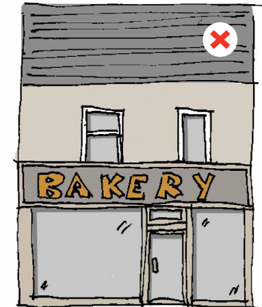
Figure 84: Poor window design and proportions, shopfront window out of scale.
