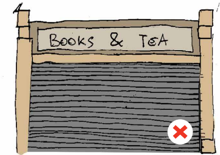
Figure 85: Roller shutter detract from the streetscape providing no visual detail.
